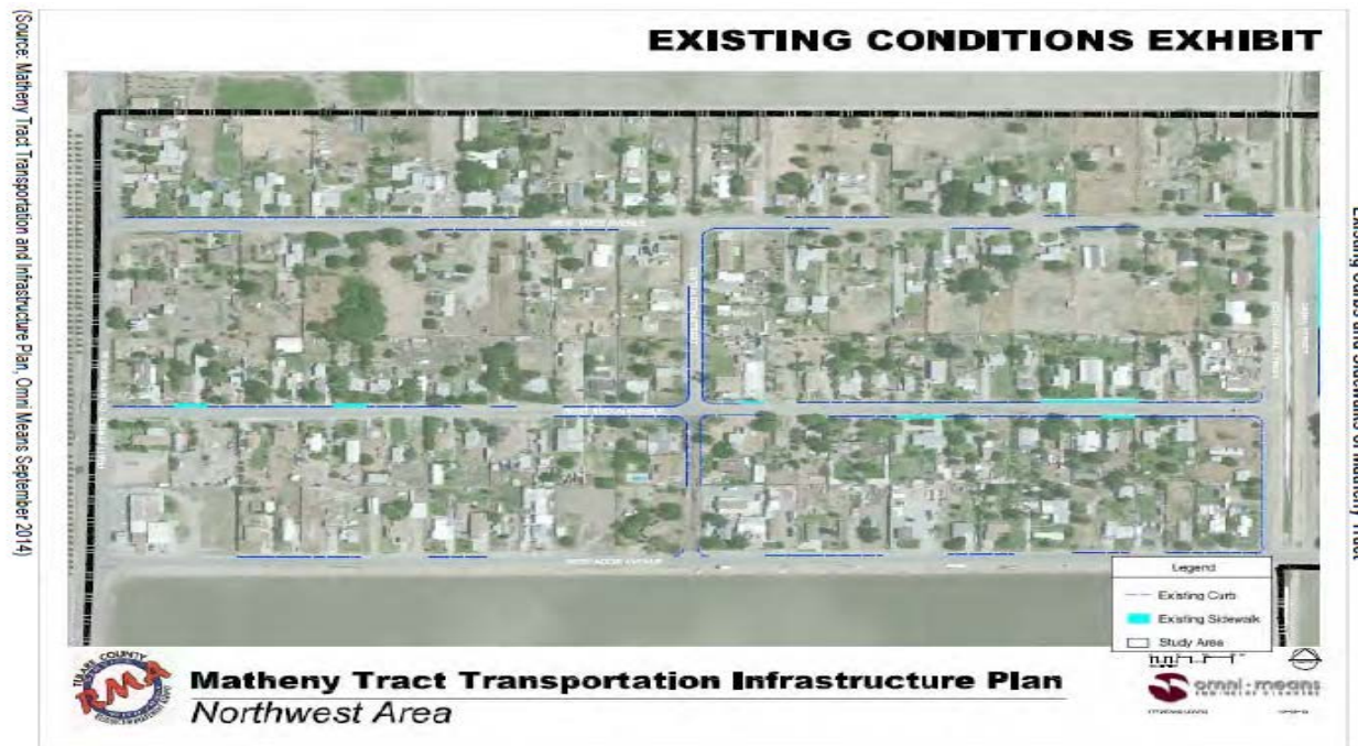
Figure 13 - Existing Curbs and Sidewalks of Matheny Tract (Northwest Area)
